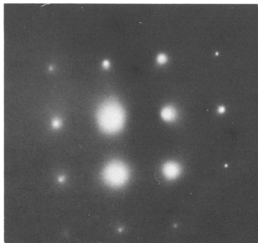
Figure 9 Electron diffraction pattern showing diffuse halo around the main spots due to GP zones.
